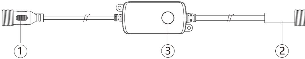
1 : Input voltage: DC12V 2 : LED light connector
